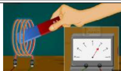
Fig: 3.5 A moving magnet produces electric current
